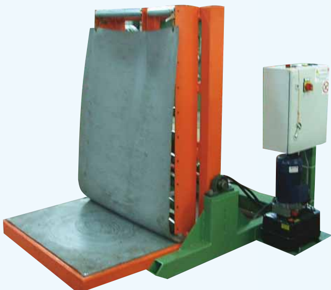
Forma ad espansione per bobine a lastra Expansion shape for LV transformer coils
